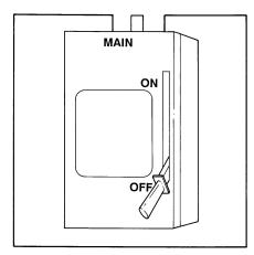
Fig. 4—Main Electrical Disconnect
